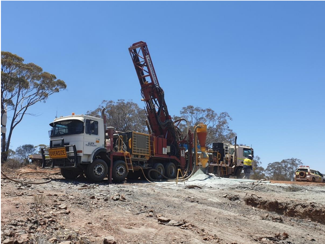
Image 1 – RC Drilling at Kangaroo Hills Lithium Project
