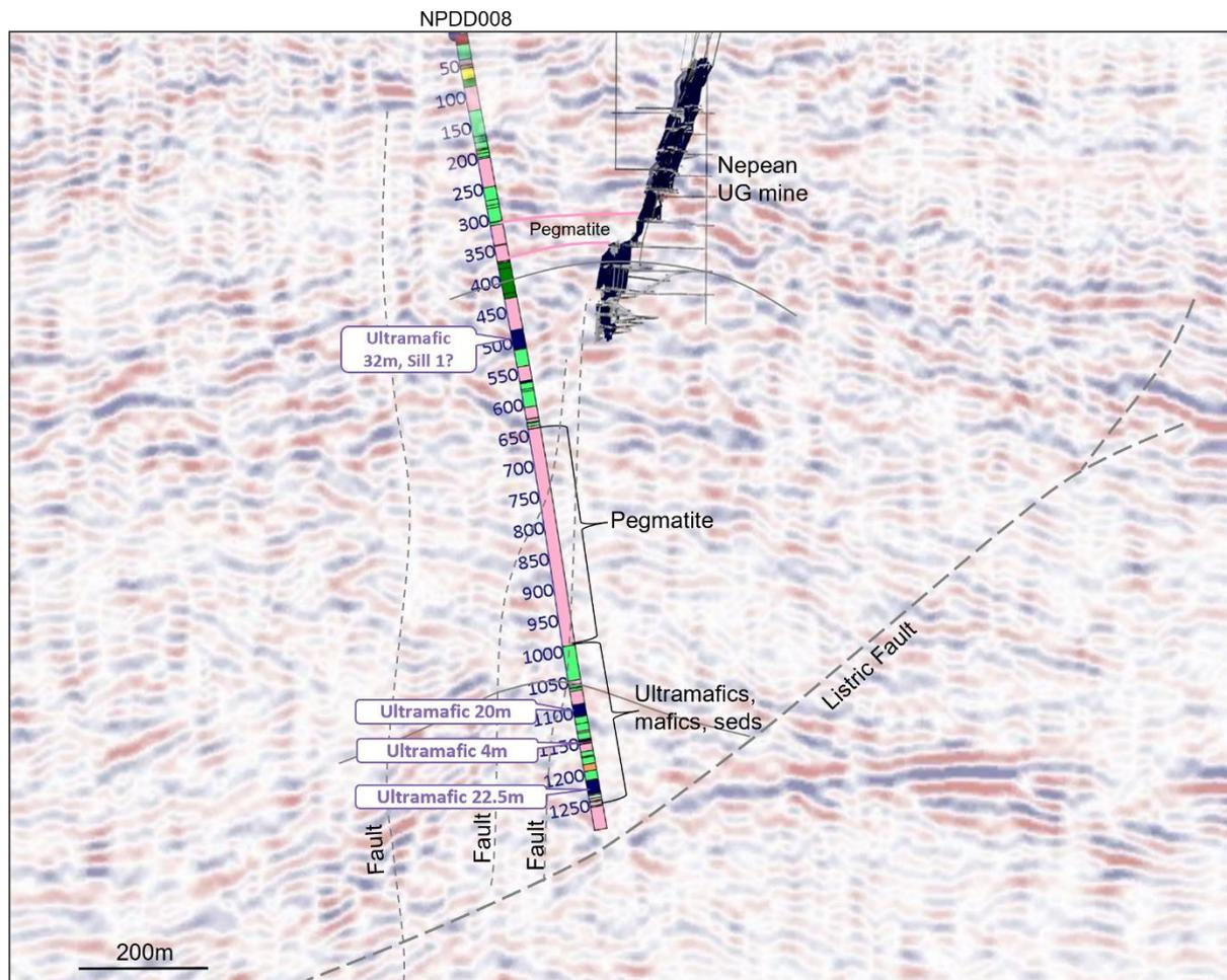
**Figure 1 – Cross section of diamond hole NPDD008 drilled below the historic Nepean mine workings showing lithologies intersected, including multiple ultramafic units, against a 2D seismic survey section. The thick pegmatite intrusion below the mine corresponds with an area of weaker reflectors, while greenstone sequences generally have stronger reflectors**
