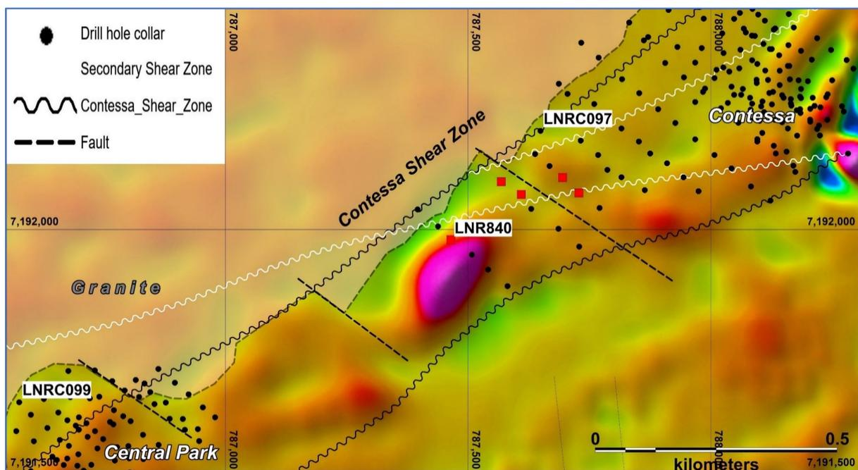
Figure 1 Contessa shear zone, bullseye magnetic anomaly to be tested by RC drilling. Adjacent transition zone gold anomalies in aircore drilling (shown as red dots). Aeromagnetic image RTP2VD, MGA94 Zone 50.
