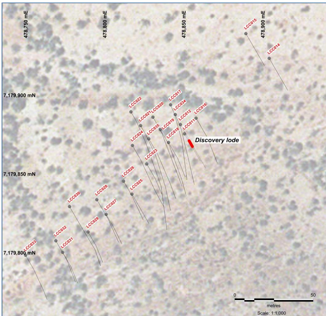
Figure 2 Collar Plan Big Sky RC Drilling (MGA94).
