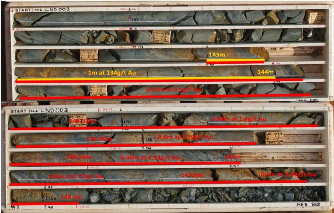
Figure 6 Contessa - mineralised core from LND003, partly oxidised and strongly sericite altered diorite.
