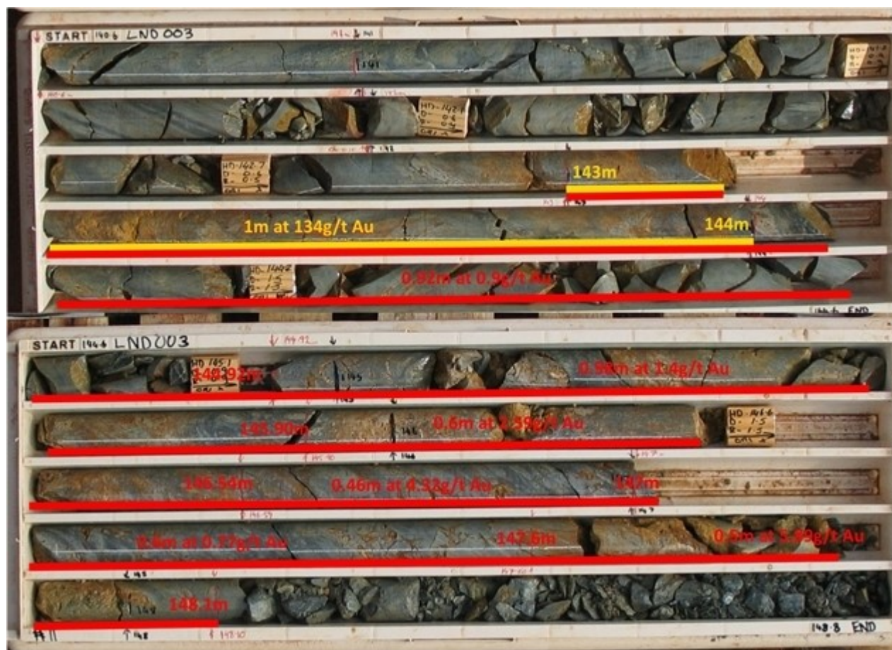
Figure 2 Contessa drill core from LND003 reporting high-grade gold mineralisation. Sample intervals and reported gold grades shown.
