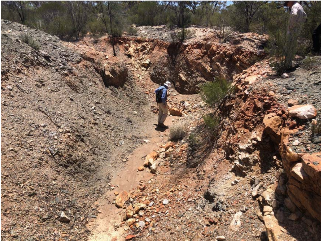
Figure 3 Costean exposing quartz veining (E15/1813).
