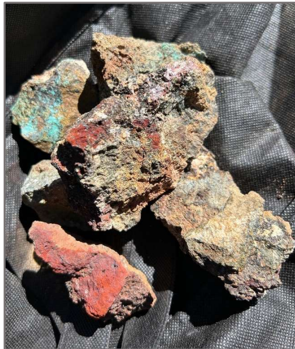
Figure 4: Rock chip sample 35, which assayed 4.25 g/t Au, 2.50% Cu and 22.7% Fe.
