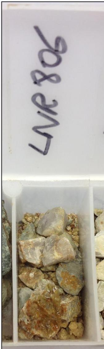
**Figure 1. Photograph of end of hole sample from LNR806 (98-99m) within intersection of 3m at 1g/t Au from 96m, quartz and quartz-feldspar-sericite vein material.**
