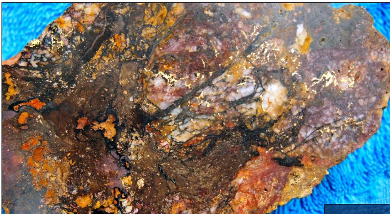
Figure 3 Visible gold in polished specimens of laterite duricrust, Marymia E52/2734. These samples were collected as specimens, have not been submitted for assay and no attempt was made to estimate the gold content.
